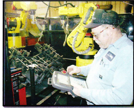
State of the art robotic welding system.
